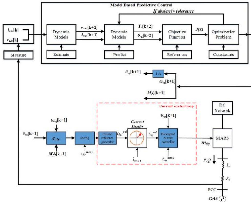
**Figure 1b MBPC-based oversight for the MARS structure**
