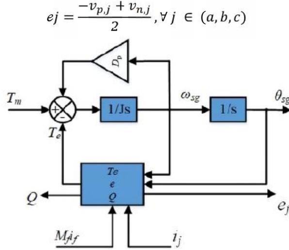
**Figure 7. Virtual Synchronous Generator control block**
