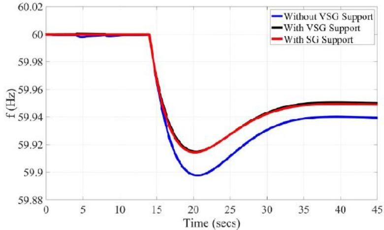
**Figure 10. Grid Regularity feedback for “LOG” at “WECC” for “SCR” is ten**
