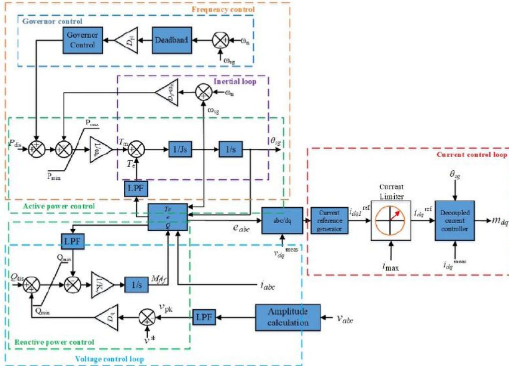
**Figure 4. Virtual Synchronous Generator-based oversight algorithm**
