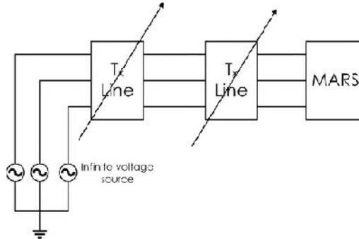
**Figure 9. Setup of the simulation model for the low “SCR” Test**
