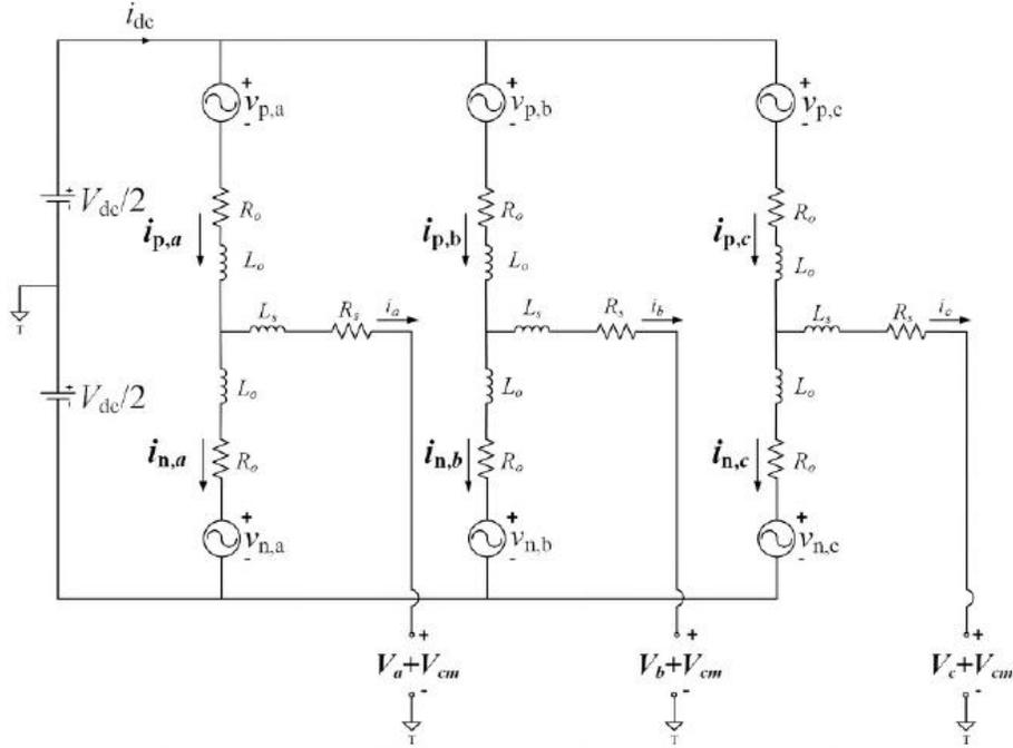
**Figure 6. Schematic of the MARS reduced model**
