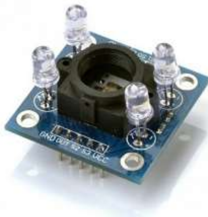
Figure 1.3 Color Sensor (Aidil, 2016)
