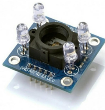
Figure 1.3 Color Sensor (Aidil, 2016)
