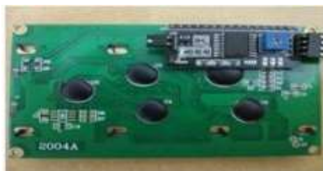
Figure 3 I2C LCD 2004 backside view
