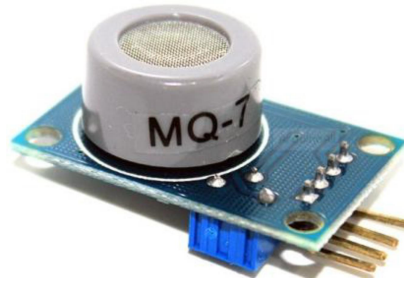
Figure 1.4 Physical Form of the MQ-7 Gas Sensor
