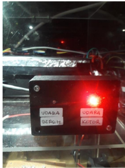
Figure 1.14 The LED lights up red when there is cigarette smoke in the room
