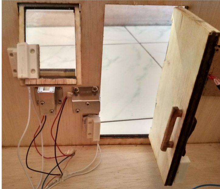
Figure 4.8 Magnetic sensor switch for normally open doors and windows
