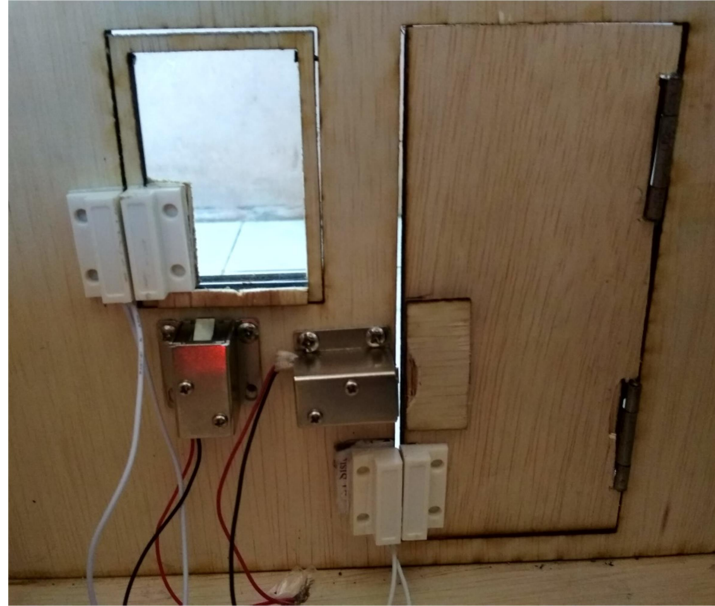
Figure 4.6 Door and window open solenoids
