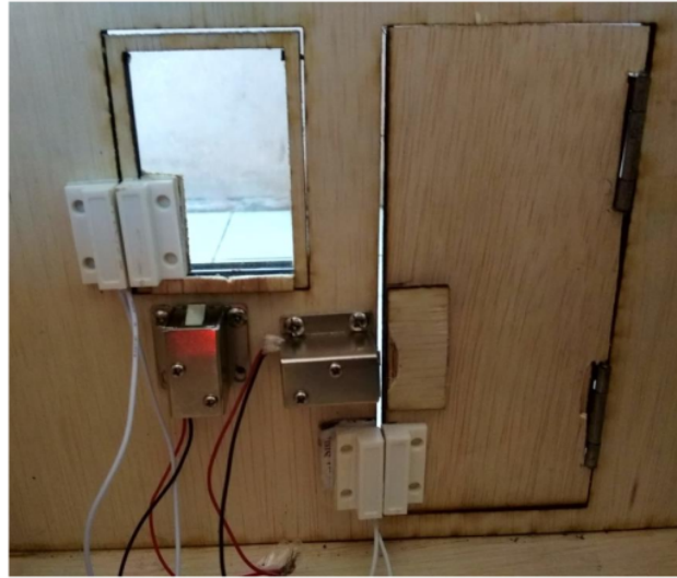
Figure 4.6 Door and window open solenoids
