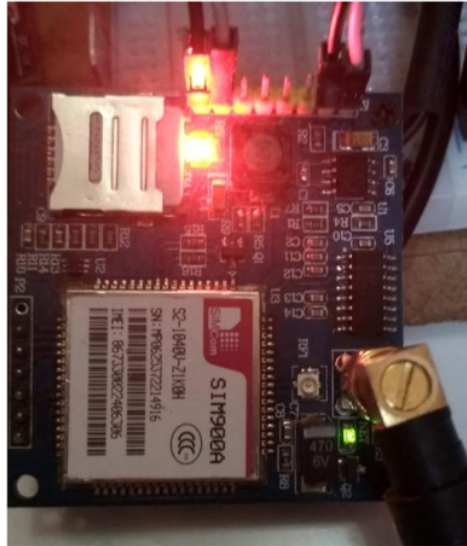
Figure 4.1 4 Sim900A gets a signal
