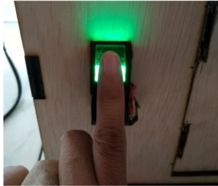
Figure 4.4 Unregistered fingerprint test
