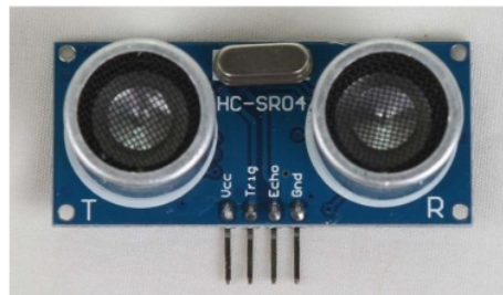
Figure 2.4 Ultrasonic Sensor ( Source: Subandi 2009)
